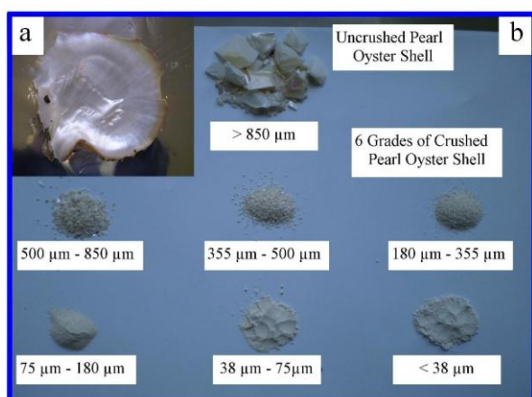
Figure 2. (a) Pinctada Maxima (pearl oyster) shells and (b) Various grades produced after sieving \text{CaCO}_3 powder (38 to 850 micrometers).
