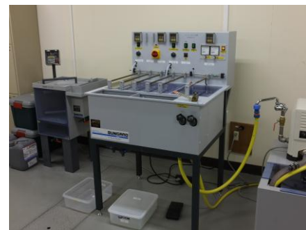
(b) Through-hole plating line (center) and Spray etching machine (left) (Compacta 30 and Splash, Bungard Elektronik)
