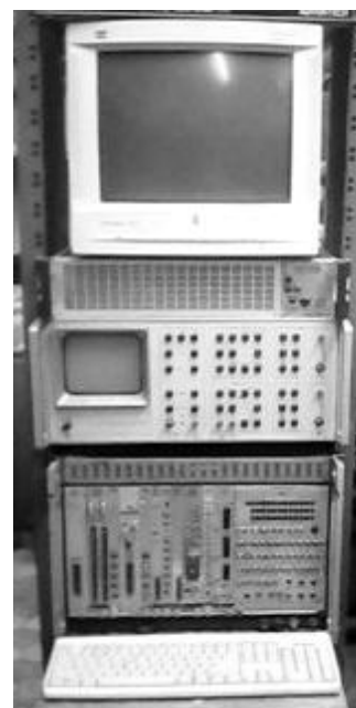
Figure 2. The earliest CAMAC-based descriptometric complex (hardware was assembled in the 1980-1990; new measurement technique ideology was proposed and new software program was written in the 2000s by «O.V. Gradov student subgroup»).
