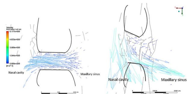
Figure 6. Velocity vectors in the anterior (left) and posterior (right) ostia at peak expiration
