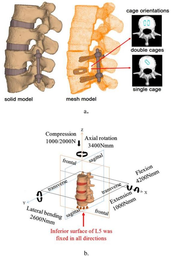
Figure 1. (a) Simulated PLIF model with PI; (b) Loads and boundary condition.
