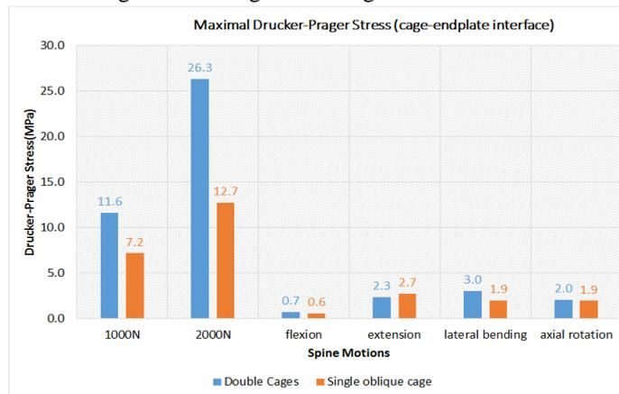
Figure 3. Maximal Drucker-Prager stress distributions at cage-endplate interface.
