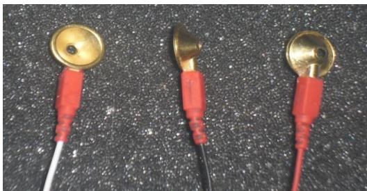
Figure 3. EEG electrodes (Source: Compiled by the authors.)
