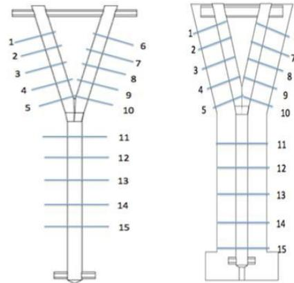
Figure 5. Transverse sections of internal and external mold for measurement.
