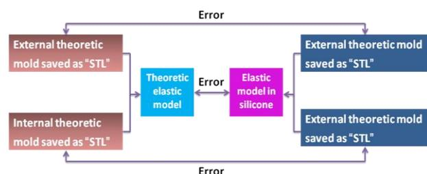
Figure 1. Protocol scheme of comparison for estimating the errors during the manufacturing process of the elastic carotid models.
