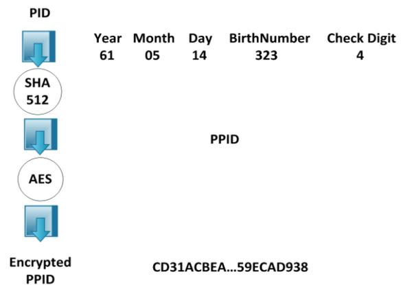
Figure 1. PID pseudonymization through a two-level hashing mechanism to provide the functionality for joint queries over different data sources.
