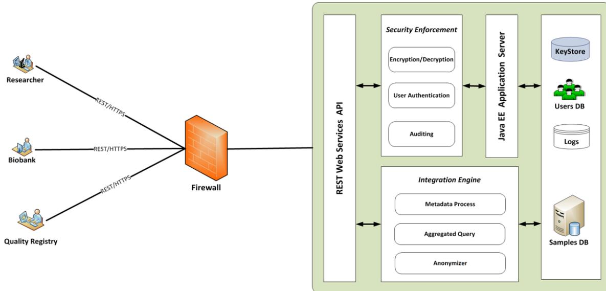
Figure 3. Overview of the eCPC integration server that is protected with firewall to filter the ingoing/outgoing traffic.
