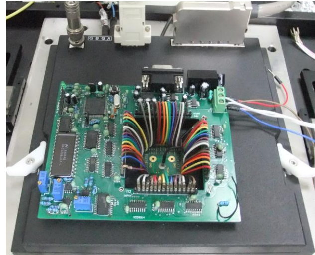
Figure 8. Implementation of the stimulator system including the pre-amplifier of the existing recording system.
