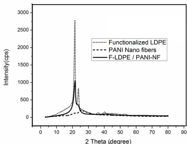
Figure 2. X-ray Diffraction of functionalized LDPE, PANI nanofibers and their blend are compared in a graph.
