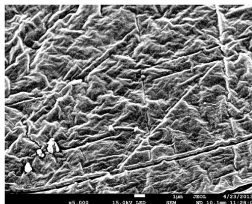
Figure 4. FESEM images of functionalized LDPE and PANI nano fibers composite with magnification of 5k times.
