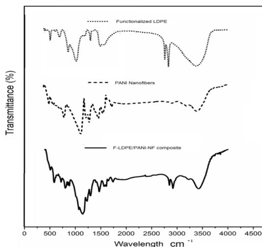
Figure 1. Fourier Transform Infrared Spectroscopy of functionalized LDPE, PANI nanofibers and their blend are compared in a graph.
