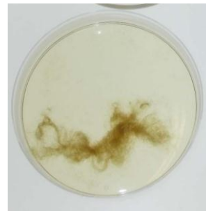
Figure 3. Result from degumming process by using 0.01 M NaOH which well corresponded with releasing fine fibers
