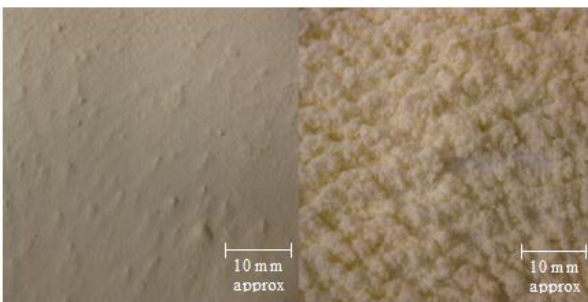
Figure 2. Filter cake appearance: SMP at left, MPC at right
