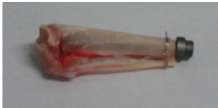
Figure 2. Amputated tibia with implant for measuring SGPZP.
