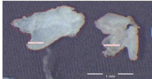
Figure 7. Particle characterization by figure analysis. The analysis function fitted polygon shows the contour of the particles.
