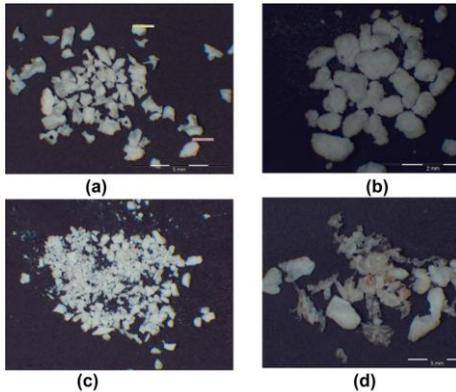
Figure 1. Commercial particles (a) Bio-oss, (b) Cerasorb, (c) Bionnovation hydroxyapatite and (d) Human bone particles from cosme and damian bone and tissue bank. scale shows 2 mm.
