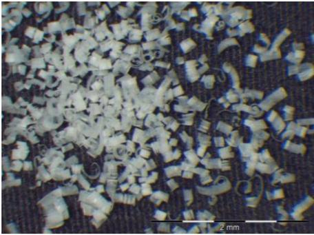
Figure 4. Typical geometry of particles obtained by turning
