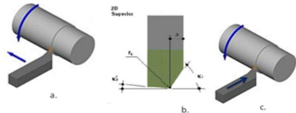
Figure 3. (a) Traditional turning process, (b) Superior 2D view of the cutting tool where  $K'r$  is the incidence angle we varied, (c) Traditional buckling process
