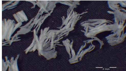
Figure 6. Typical geometry of particles obtained by buckling.
