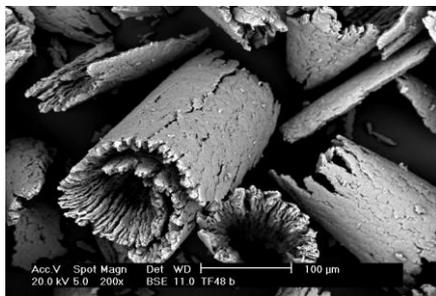
Figure 2. SEM of spiral bone particles at 200x.
