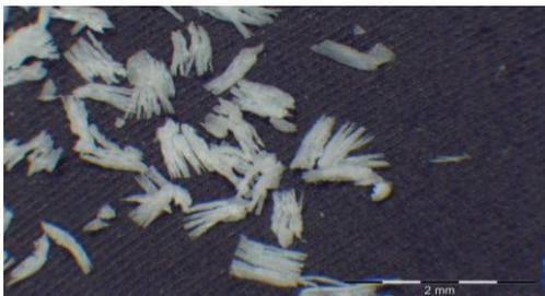
Figure 5. Typical geometry of particles obtained by turning with an incidence angle
