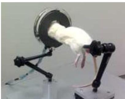
Figure 3. Si-PM based PET during measurement of rat brain
