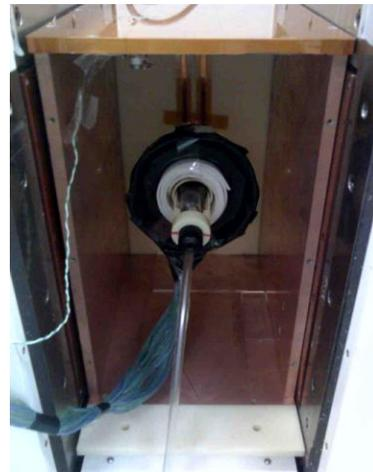
Figure 4. Si-PM based PET during simultaneous measurement with 0.15T MRI
