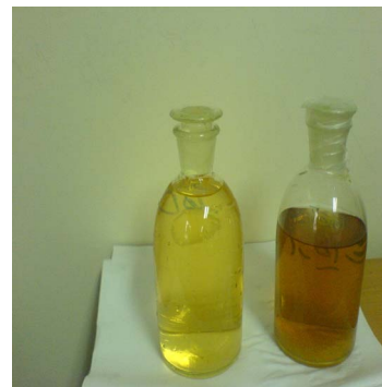
Fig. 10. The effluent visual properties before ( right bottle )and after bio-enzyme batch reactor (left bottle)
