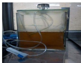
Fig. 1. The batch bioreactor (experimental conditions: 25 ^{\circ} C, pH: 6-9, reaction time: 1-10 days)
