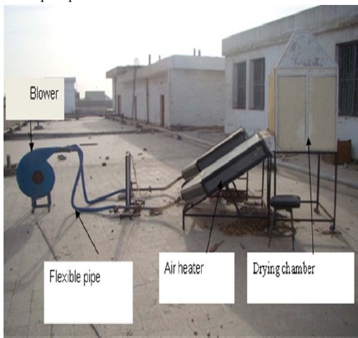
Fig. 1. (a) A schematic diagram of the experimental set-up. (b) Photograph of the experimental set-up.
